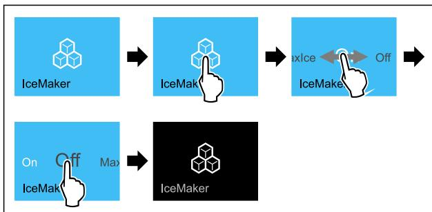
Fig. 48 Example illustration of the active IceMaker function
