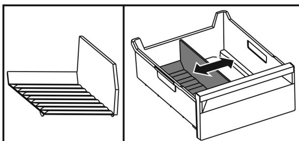
*Fig. 115 Example illustration of the ice compartment divider*
