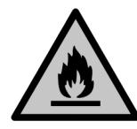
This symbol is located on the compressor and indicates the danger of flammable materials. Do not remove the sticker.
