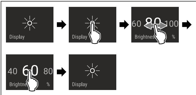
Fig. 55 Example illustration: Switch from 80 % to 60 %.
