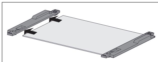
Fig. 129 Glass shelf with retaining part
